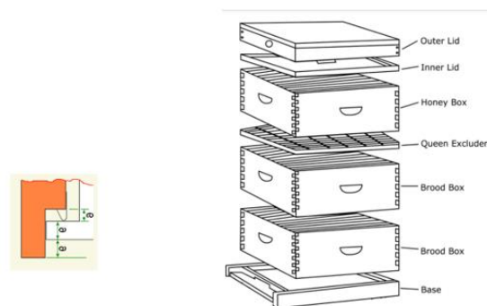
Fig.3.1 Components of a standard beehive
